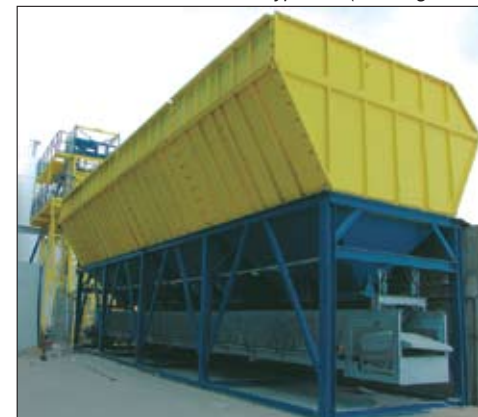
Silo en fila row type silo (above ground)
