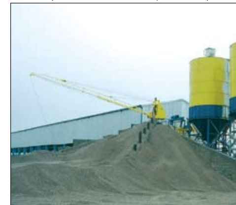
Almacén pluma arrastre star bin/boom scraper
